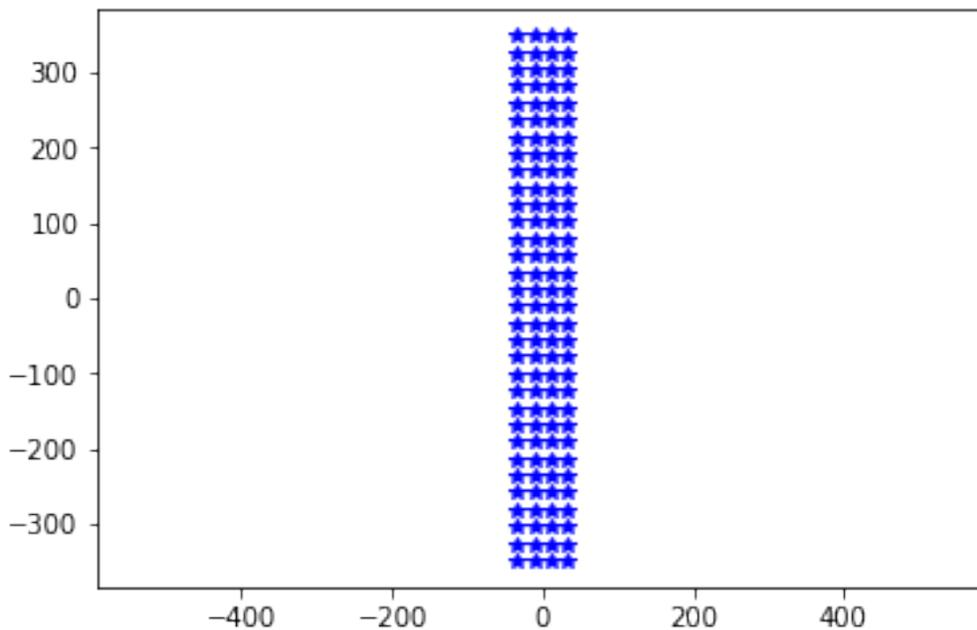
By default the MEA is instantiated with its center of mass at (0,0,0) and electrodes lying in the plane specified in the yaml file (by default plane is yz)
