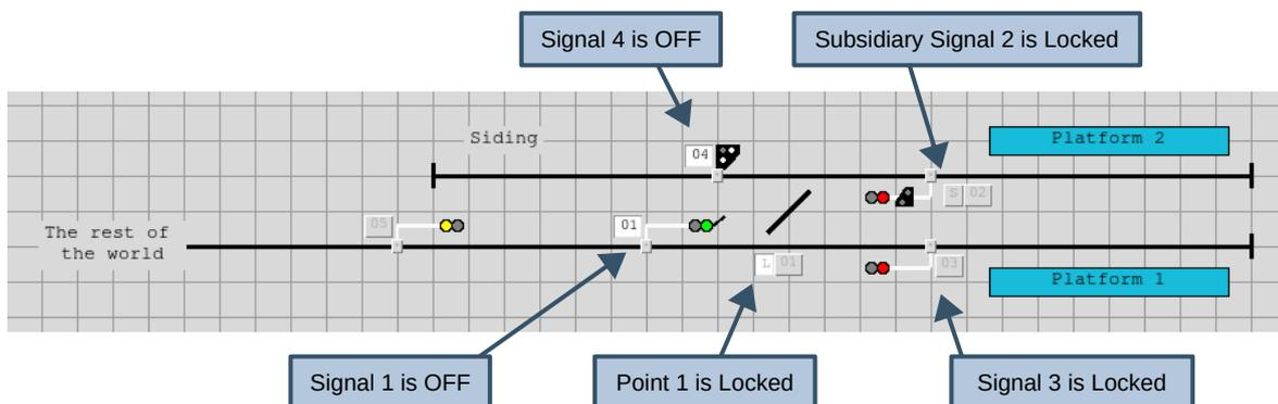
Once all signals have been returned to 'ON' then the points can be changed to test the other signal routes. Click on the 'L' button to 'release' the Facing Point Lock (FPL) and enable the main point control button. The point can then be switched .
