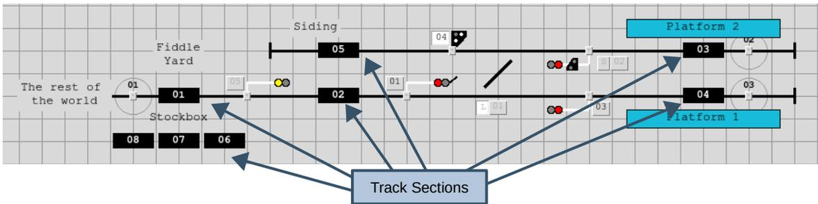
Each signal then needs to be edited to define the track section 'behind' the signal (i.e. the track section that would be 'cleared' when the signal is passed) and the track section 'ahead of' the signal (i.e. the track section that would be set to 'occupied' when the signal is passed). For signals controlling multiple routes, the track section 'ahead' needs to be defined for each route. This configuration is defined via the **Automation** tab of the signal configuration dialog.
