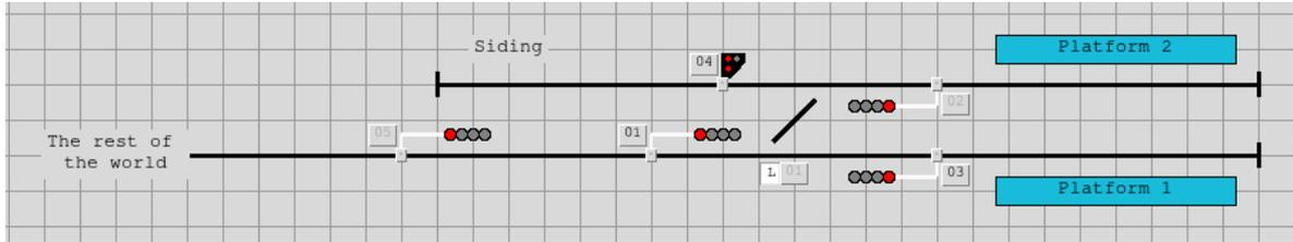
To signal the train movements we have defined, we need to edit Signal 1 to provide a route indication (to differentiate between the routes into Platform 1 and Platform 2). At the same time, we'll change it to a two-aspect signal and configure the DCC addresses. As before, **double-left-click** to bring up the configuration dialog and use **Apply** or **OK** to save the changes
