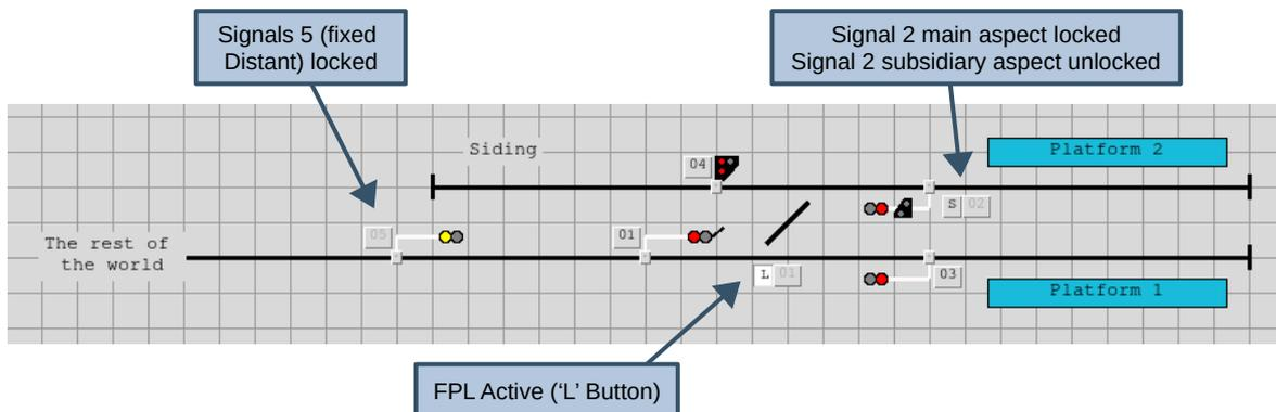
In this state, the interlocking with conflicting signals can be tested. If Signal 4 is switched 'OFF' then the subsidiary aspect of Signal 2 will be locked, and vice versa. Similarly, if signal 1 is switched 'OFF' then Signal 3 will be locked, and vice versa. Note that when a signal is set to 'OFF' the points are locked and cannot be changed until the signals are returned to 'ON'.
