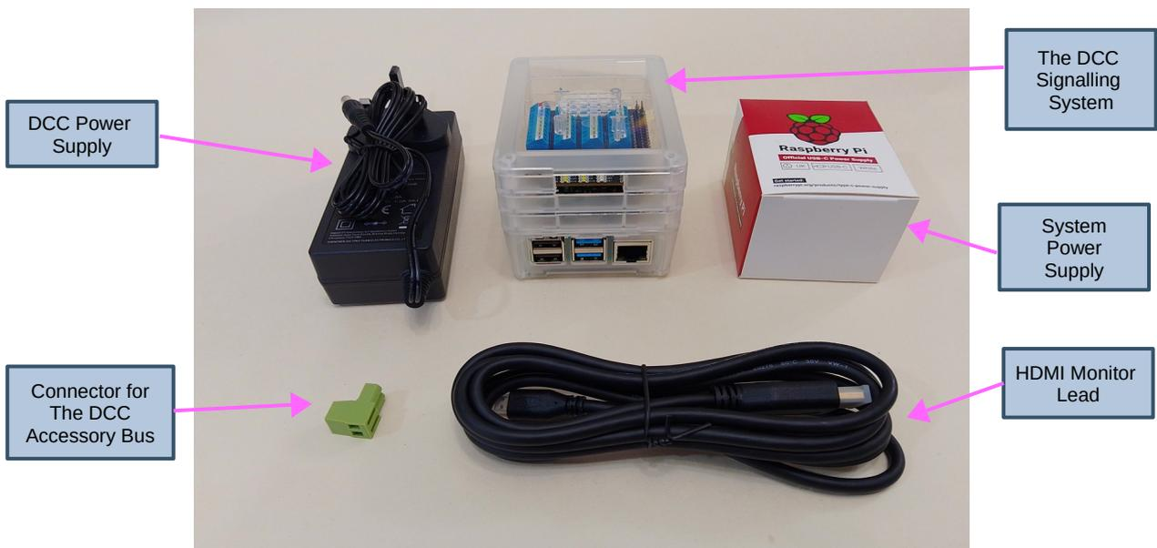
**Before proceeding, inspect all of the components carefully for damage (especially the power supplies). If you suspect damage then contact DCC Model Railway Signalling immediately to arrange an exchange (see <https://www.model-railway-signalling.co.uk/> for contact details).**
