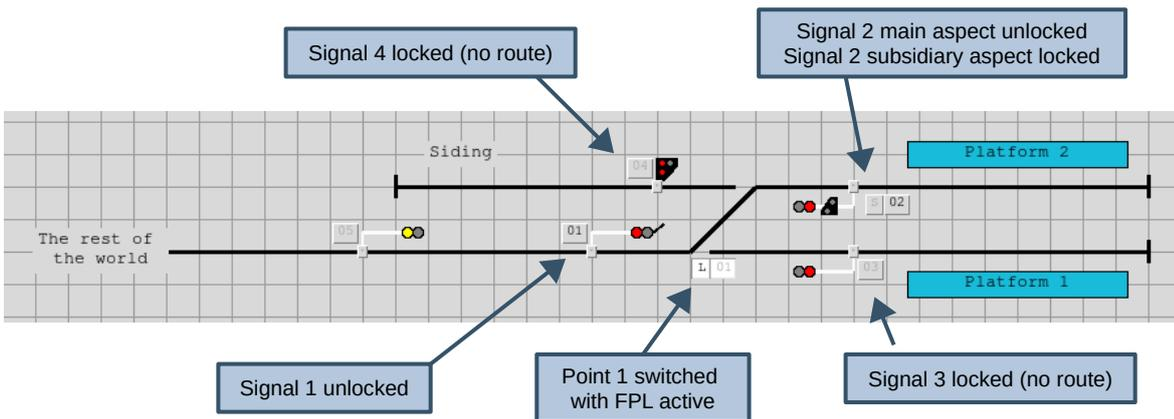
The interlocking with conflicting signals can now be tested in this configuration. If signal 1 is set to 'OFF' then Signal 2 will be locked and vice-versa. Note that when Signal 1 is 'OFF' it will display the appropriate route indication (in this case a left hand feather).
