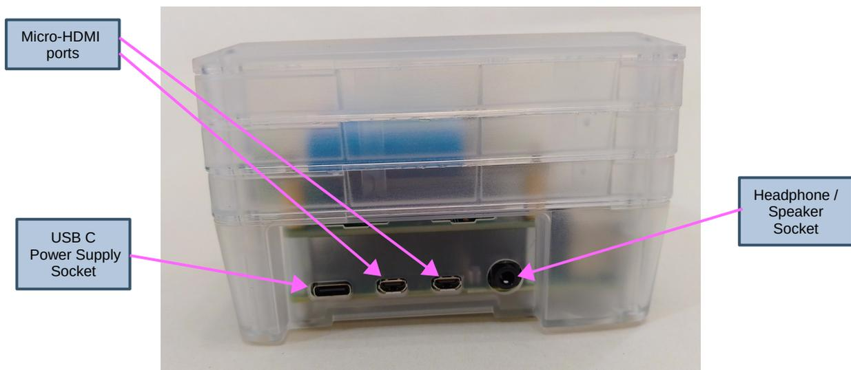
**Only ever use the power supply that comes with the system (or another official Raspberry-Pi USB-C power supply) – use of non compatible power supplies may damage the system.**
