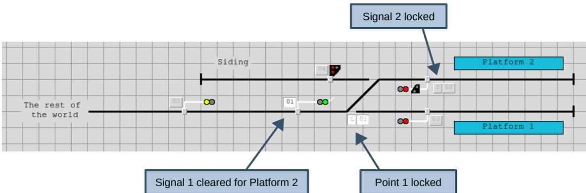
Although interlocking is defined via the signal configuration dialog, the resultant Point interlocking can be viewed (as read only) via the **Interlocking** tab of the point configuration dialog. This shows all the signals/routes which (when cleared for a movement) would lock the point.
